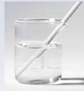
The light refraction indices of the monomer and the glass rod are different.
