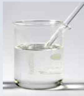
The light refraction index of the monomer corresponds to that of the filler, the glass rod in this case.
