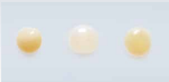
Starting situation: Tetric EvoFlow (left), SDR Flow* (middle) and Palfique Estelite LV* (right) have been applied to a vertically positioned glass slab. Source: Ivoclar Vivadent AG, Schaan, 2012
